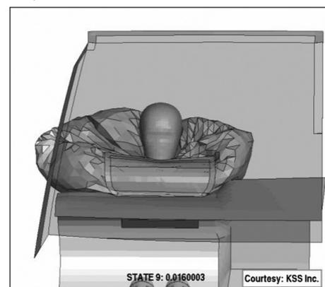
Figure 2. Airbag simulation
